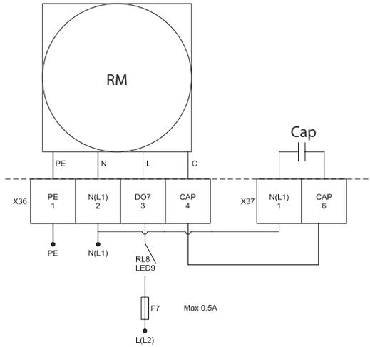
RM - Rotorantrieb; Cap - Kondensator
