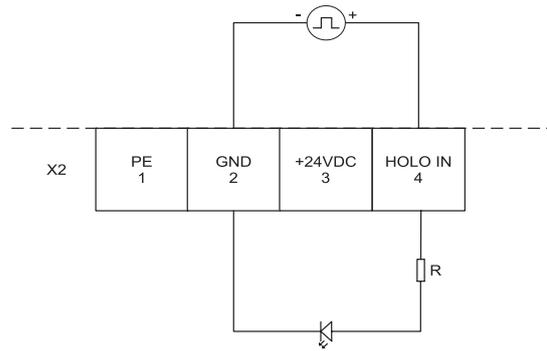
$R = 1 \text{ k}\Omega; U_f = 1,5 \text{ V}; I_{f, \text{min.}} = 1 \text{ mA}; I_{f, \text{max.}} = 50 \text{ mA}$
