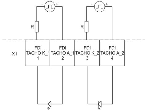
$U_f = 1,5 \text{ V}; I_{f, \text{min.}} = 1 \text{ mA}; I_{f, \text{max.}} = 50 \text{ mA}$
